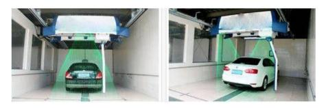
The system is equipped with advanced position sensor, ultrasonic sensor and closed loop controller to detect location and size of vehicles. The detected digit signal is sent to central control unit to adjust the washing size automatically.
